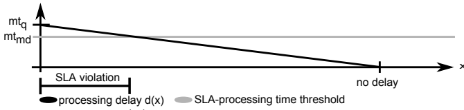
Figure 2: Processing delay d(x) based on the x -th processed event and query migration time mt_q considering the SLAs mt_{md} .
