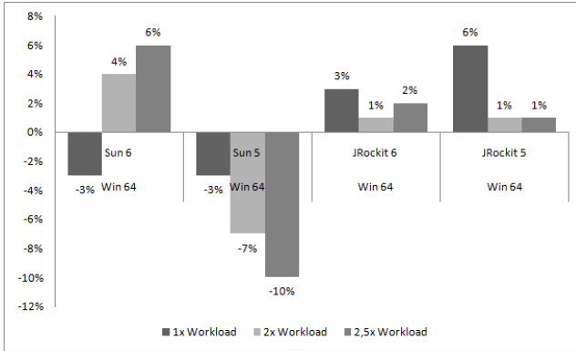
Figure 13. Penalties For Suns HotSpot and Oracles JRockit MC in Version 5 and 6, Measured on a 64bit Windows 7.
