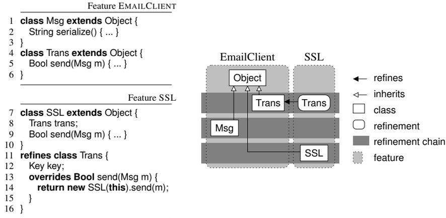
**Fig. 1.** A feature-oriented email client supporting SSL encryption.
