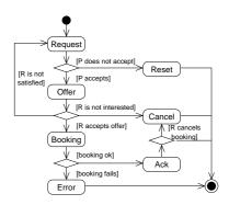
Figure 3: Message flow in the communication system
