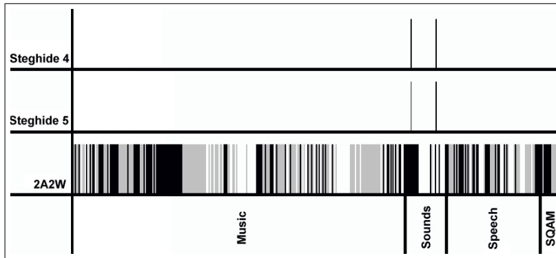
Fig. 4: Results from the transparency benchmarking for two steganography and one watermarking algorithm over a test set of 389 files. The computed |ODG| value is colour-coded in three classes: below 0.2 (white), between 0.2 and 1 (grey) and above 1 (black). (Values taken from [3])
